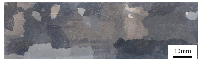
Fig. 4. Macrostructure of secondary recrystallization annealed strip.
