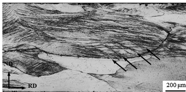
Fig. 12—Optical microstructure showing the shear bands of the first cold rolled strip (R1-FCR) which was processed by route R1.
